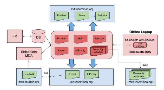
The new processing is shown as "Per-entity metadata" in the center bubble, and the new distribution layer is the "mdq.incommon.org" box in the lower right.
