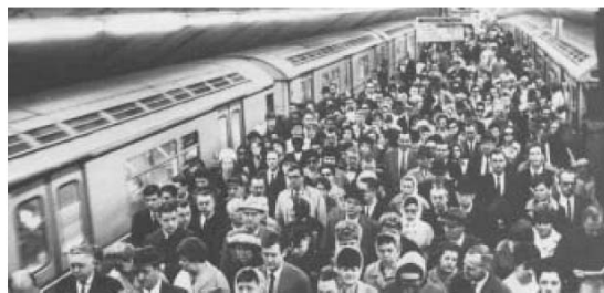
Jammed Flow (Figure from p.90 of Pushkarev and Zupan: space per pedestrian is about 0.35 \text{ m}^2 – on the lower end of the speed-flow curve).
