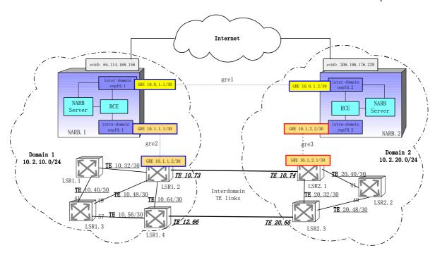
Figure 6: An example network configuration with NARB in a two-domain environment.
