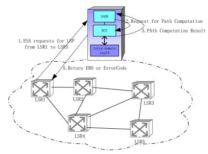
Figure 2: NARB use case in a single-domain network.
