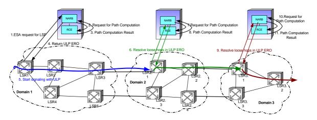
Figure 4: Illustration of the ULP-based inter-domain path computation.
