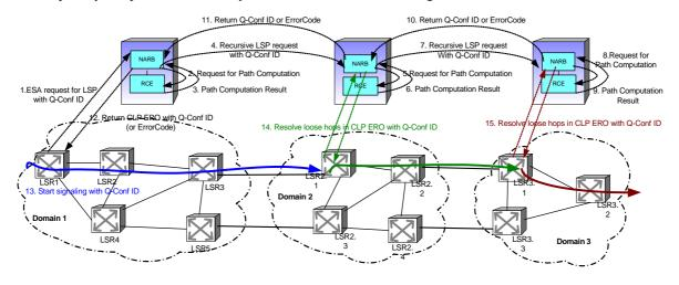
Figure 5: Illustration of the CLP-based inter-domain path computation.
