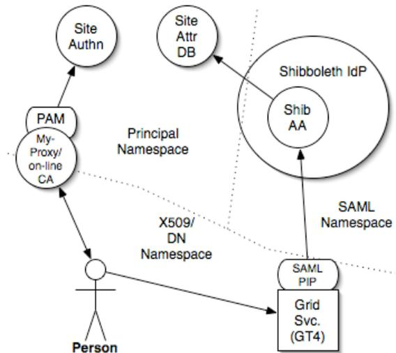
**Figure 4: Different namespaces involved in an integrated MyProxy/Grid Service/Shibboleth transaction. The principal name used for authentication (at left) must be transmitted and used for attribute retrieval (upper right).**
